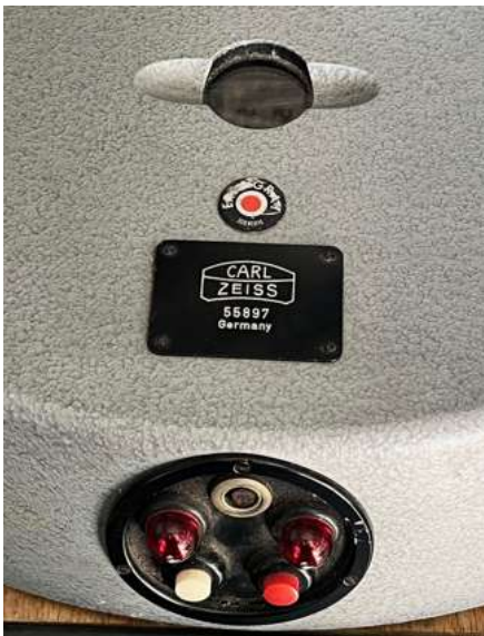
Power supply for shutter, exposure meter and front control panel (below).
