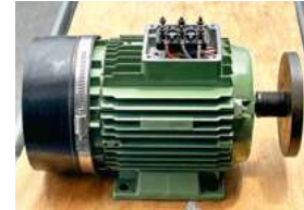
Emco Super 11 main single phase motor
