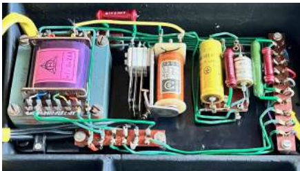
Power supply for shutter, exposure meter and front control panel (below).
