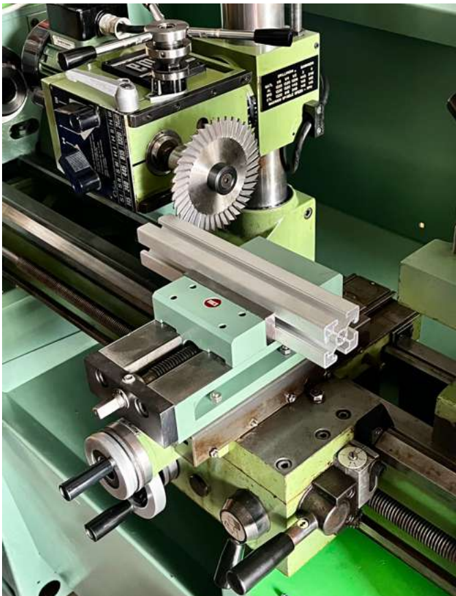
Cutting an Aluminum block with a 5" circular saw with cross feed. Right, two automatic feed controls in Emco Super 11
