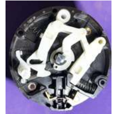
Inside Power Switch
