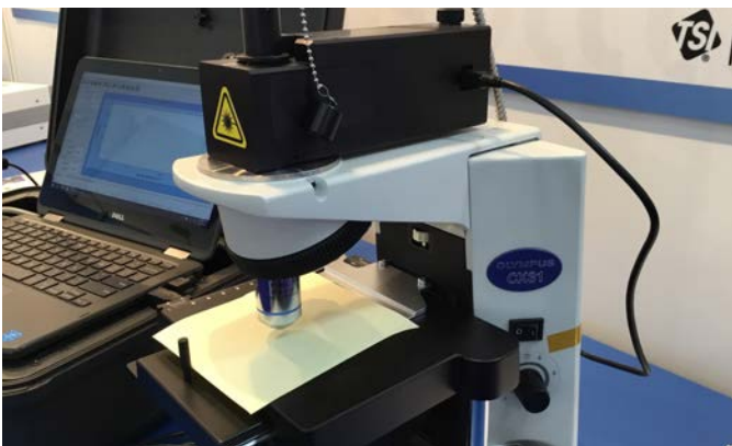
28. Soliton Raman microscope uses back illuminated CCD sensor, and dual 532 nm, and 785 nm laser. Its compact/portable package can be mounted on various microscope brands. Email: w.wagner@soliton-gmbh.de
