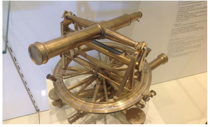
Two types of equilateral telescopes utilized for early clock accuracy. A star was centered in its reticule, and after 24 hours, the star had to reappear on the same spot (actually minus 4 minutes due to the earth's rotation around the sun).
