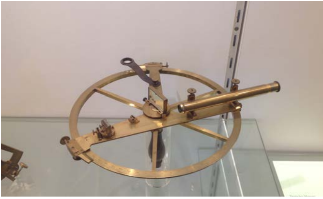
An early theodolite made of brass utilizes first surface mirrors, a Galilean telescope, and graduated angular scale.
