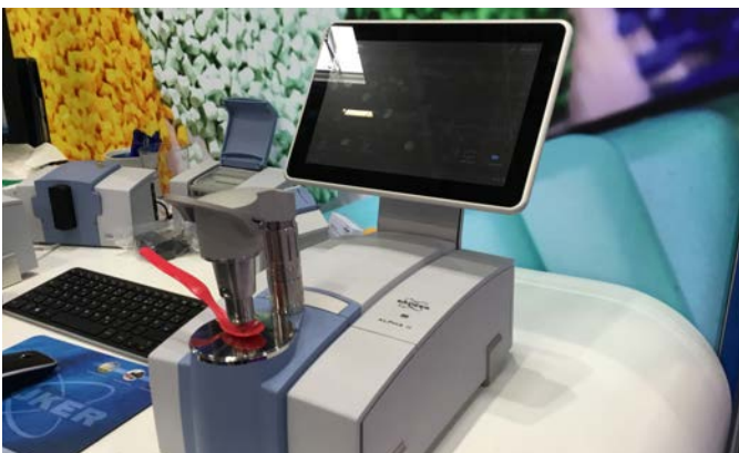
13. Two desk top analyzer workstations by Bruker offer menu driven rear mounted touch display (left), and monitor/instrument door closure combination (right) to save desk top space. Email: jurgen.sainwatzki@bruker.com
