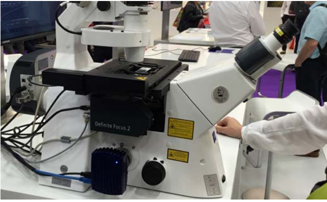
23. The basic Zeiss inverted microscope design (left) with added LSM 800 galvo scanning module (right) is mechanically challenging. Although both units are sitting on an optical table, their optical alignment requires slight mid floating point.
