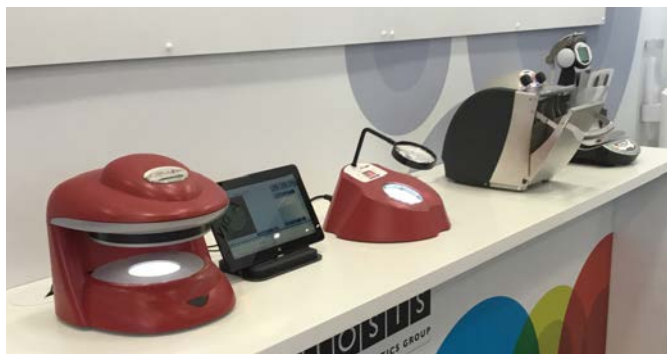
3. Peri dish observation station by Synoptics. Simple but very useful idea that allows image capture, measurement, and visualization of petri dishes with viewing comfort, and image enhancement. Email: jayne.arthur@synoptics.co.uk
