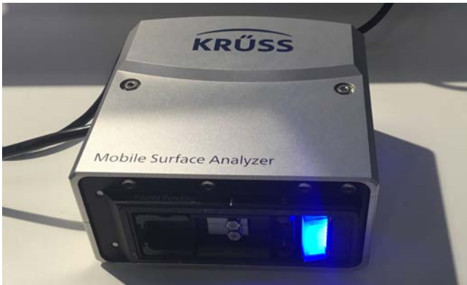
47. Contact angle measurement (by a liquid drop) is accomplished by this compact mobile analyzer for inspection in automobile parts, curved surfaces, and surface free energy measurements made by Krüss. Email: d.frese@kruss.de
