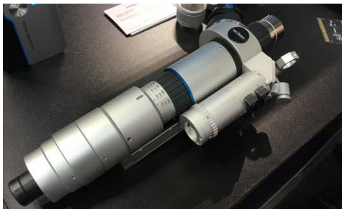
10. Digital microscopes by Hirox utilize their own in-house designed lenses for maximum resolution, and increased depth of field. Their close focus lenses (left) utilize side illumination via in-line beamsplitter. Email: emilien@hirox-europe.com
