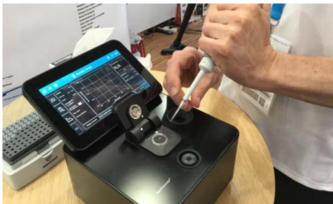
61. IMPLEN desk top microvolume spectroscope has 7" touch panel user interface to measure down to 0.3 micro liter sample volumes. The 200-900 nm photometry curve is instantly displayed (right). Email: msahiri@implen.de
