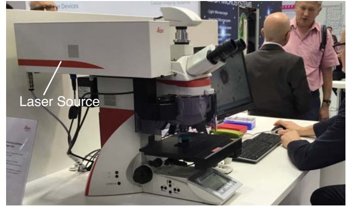
11. Leica microscopes with focusing stage automation, and motorized turret feature heavy rear end body design. The detachable X-Y stage allows its interchange with motorized stages. Email: marika.sosnowski@leica-microsystems.com
