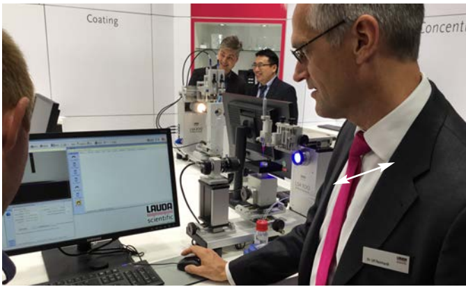
14. Contact angle measurement is handled easily with this modular system, and its computer user interface by Lauda Scientific. The software calculates the contact angle of a drop on the surface. Email: ulf.reinhardt@lauda-scientific.de
