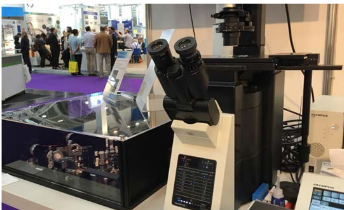
17. The tomographic or Stimulated Emission Depletion Microscopy (STED) produces images below the optical diffraction limit by using a phase plate to produce doughnut shape pulse. Watch online interview with Stefan Hell on youtube. The purpose of binocular head swinging vertical (left) is to be out of the way in a lab space: kareem.soliman@llg-ev.de
