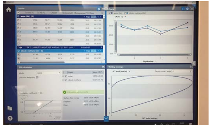
47. Contact angle measurement (by a liquid drop) is accomplished by this compact mobile analyzer for inspection in automobile parts, curved surfaces, and surface free energy measurements made by Krüss. Email: d.frese@kruss.de
