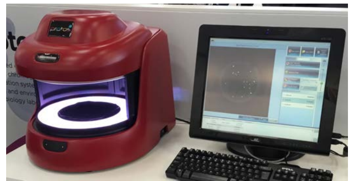
3. Peri dish observation station by Synoptics. Simple but very useful idea that allows image capture, measurement, and visualization of petri dishes with viewing comfort, and image enhancement. Email: jayne.arthur@synoptics.co.uk
