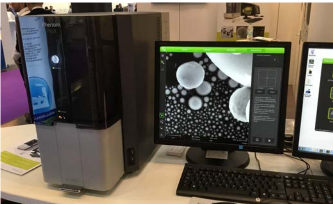
45. This high performance table top SEM by Phenom World, costs 50-100K euros. It features fully integrated elemental analysis, smooth sample navigation at up to 150,000X magnification. www.phenom-world.com
