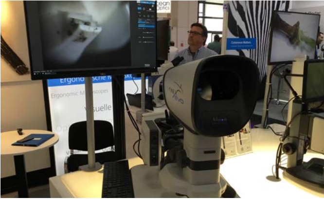
46. Vision inspection microscopes utilize reflex optics for viewing comfort. Reflex optics reduces weight just as in large astronomical telescopes. The binocular 3D viewing can be adjusted like normal scopes. Email: summer@visioneng.de
