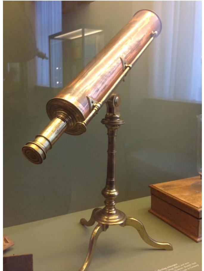
A late 1800's brass telescope with rear focusing knob to adjust main objective position via a long lead screw rod.
