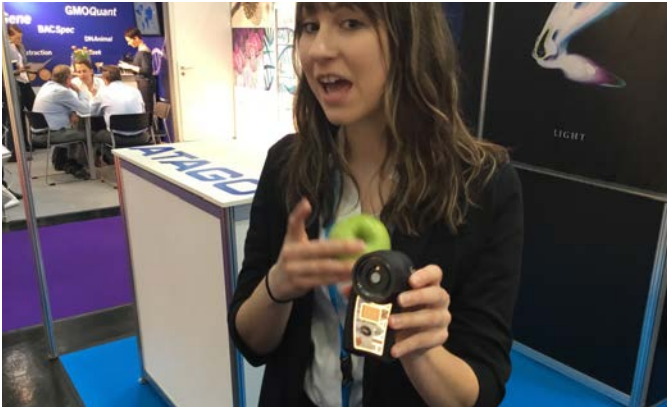
1. This apple sweetness tester utilizes LEDs to measure its interaction inside an apple to measure its sweetness. The Japanese made handheld device is pressed against an apple, and gives instant answers. Email: moriguchi@atago.net
