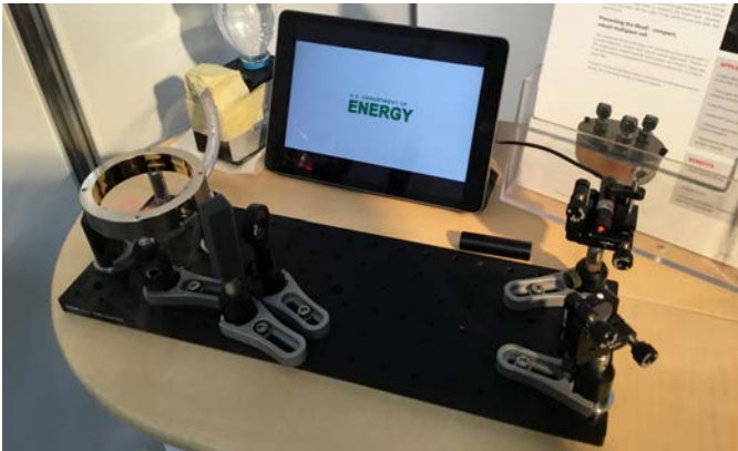
15. The IR cell utilizes a cylindrical multi-pass cell to combine the long optical path in a small detection volume for increased measurement sensitivity, and eliminates bulky cells for laser abs. spectroscopy. markus.geiser@irsweep.com
