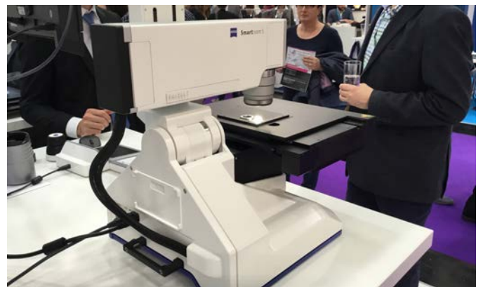
Versatile viewing of 3D objects with this Zeiss system, with adjustable angular viewing possibilities. The vertical mono rail (left) allows vertical positioning while the swivel joint (rear view, right) allows angular adjustment for oblique viewing.
