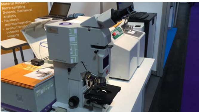
2. This slim microscope body design (left) is a wide range IR microscope (IROS) by Ostec. The microscope features all reflected optics for its wide spectral range. Right, Confocal Raman microscope. Email: pribora.v@ostec-group.ru
