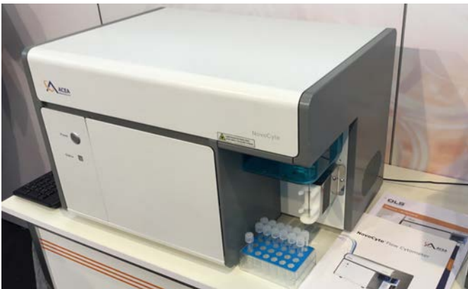
42. Complex beam layout in this flow Cytometer at OLS booth contains six PMT arrangement, two other detectors, and three laser sources to identify and analyse specific sub-populations of cells. Email: info@ols-bio.de
