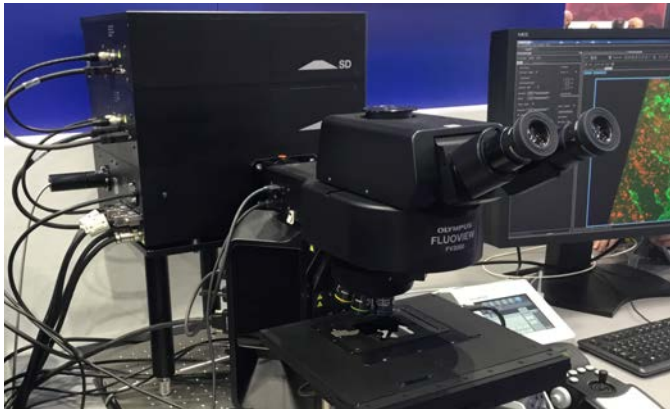
48. Olympus FV 3000 Single Photon Confocal Laser Scanning microscope uses Bicolle SD PMT detectors, highly sensitive HSD detector, Resonant, and Hybrid galvos for fast image scanning. The huge cabinets of these microscopes allows the workstation to be placed in a separate room for cooling. Email: bjorn.sieberer@olympus.de
