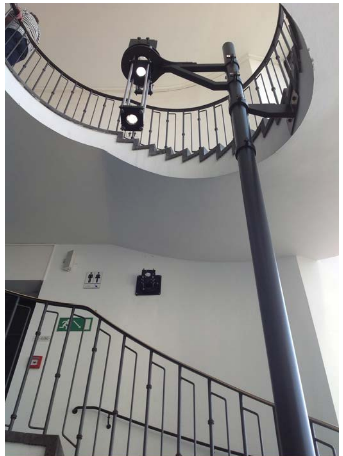
The sun telescope is beautifully designed to blend with the architecture. There is an automatic tracker mirror on top, and a lens projection system utilizing Spindler & Hoyer's Macrobench system. The image is projected on screen below.
