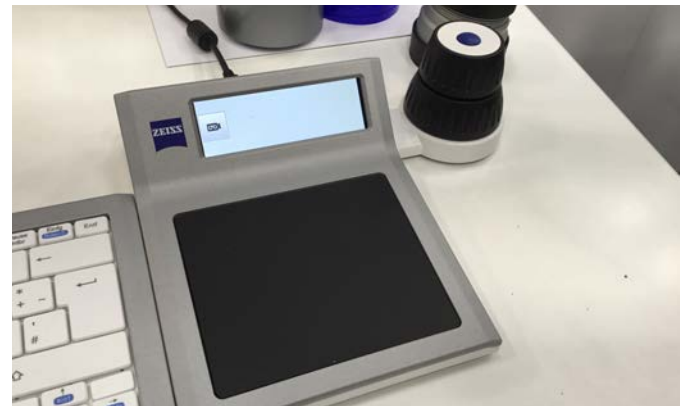
Modular specimen platform that would accept standard rectangular microscopes slides, and circular petri dish containing bacterial growth, etc. Various new touches in ergonomic control of the microscope movements, next to the keyboard.
