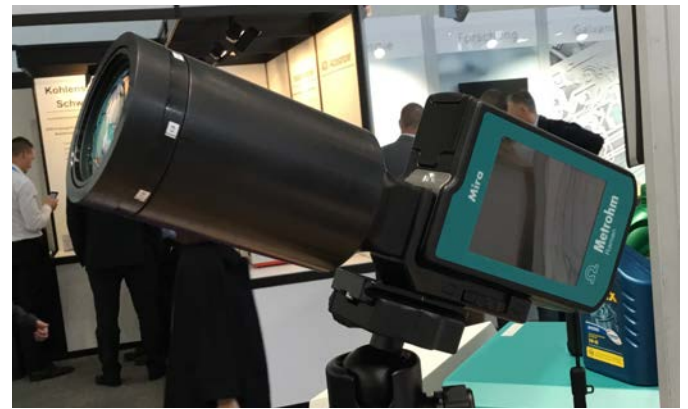
27. Well designed modular accessories for Metrohm Raman viewing device: The finely machined anodized Aluminium accessories fit together as if they are made of injection molded plastic. Email: nicolas.ruehl@metrohm.com
