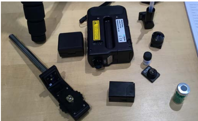
27. Well designed modular accessories for Metrohm Raman viewing device: The finely machined anodized Aluminium accessories fit together as if they are made of injection molded plastic. Email: nicolas.ruehl@metrohm.com
