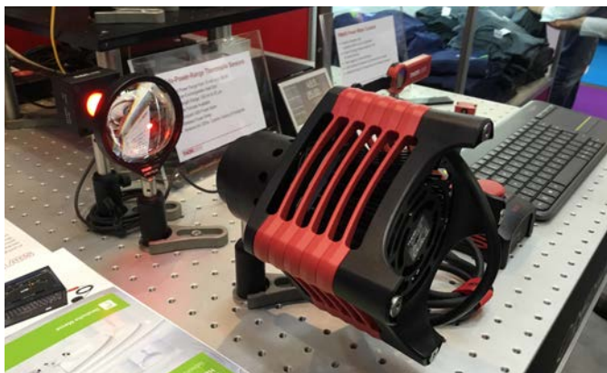
16. Thorlabs SOLIS narrowband LED light source for fluorescence microscopy is capable of outputting from UV to near IR. Various models with center wavelengths: 365, 385, 405, 445, 525, 623, and 850 nm: shallwig@thorlabs.com
