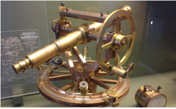
Two types of equilateral telescopes utilized for early clock accuracy. A star was centered in its reticule, and after 24 hours, the star had to reappear on the same spot (actually minus 4 minutes due to the earth's rotation around the sun).
