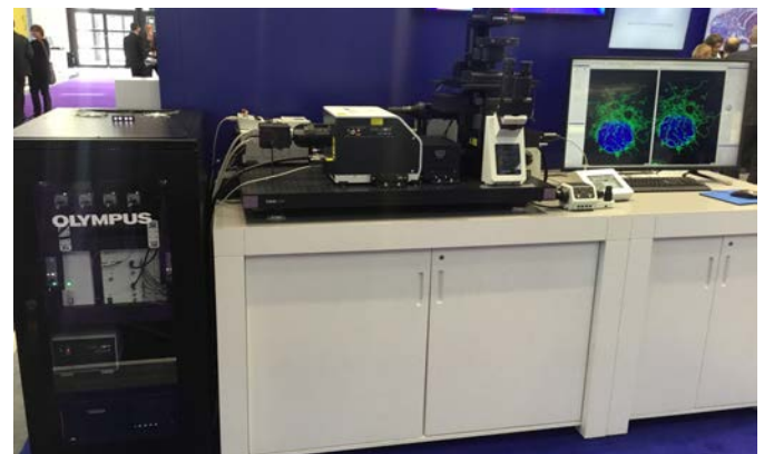
48. Olympus inverted Spinning Disk microscope claims to deliver 120 nm resolution (above right) compared with 280 nm limit of traditional microscopes. It utilizes Yokogawa CSU-Wi 4000 rpm Nipkov disk with six light sources: 405, 488, 551, 640, 515, and 445 nm, and IXplore spinSR for image enhancement. Email: bjorn.sieberer@olympus.de
