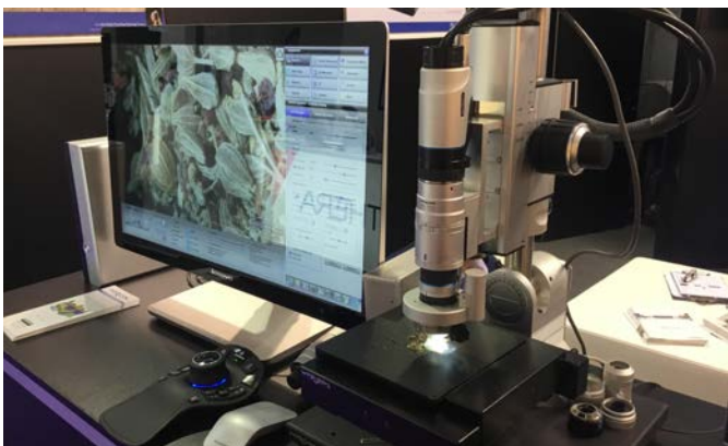
50. Hirox high resolution optics utilizes in line illumination, and rotating mirror 360 view of the sample with long depth of field. They offer interchangeable optical heads plus variable angle support column. Email: emilien@hirox-europe.com
