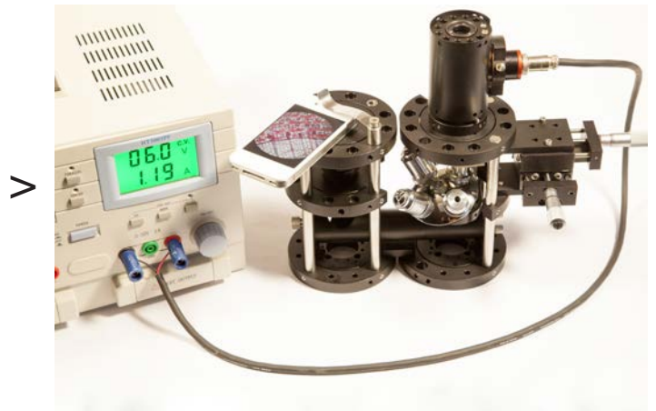
Various microscope designs constructed with Optoform Cage System.
