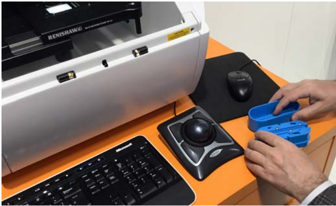
29. Above-left, Rainshaw's Raman microscope in standard package. Right, their RA802 pill examination machine displays a cross sectional slice of the pill, and its inner contents. With cool easy to use clever tool (lower left), the pill is first sliced in half. The distribution of pill contents are displayed (above-right), and thanks to image processing software, their comparative cross sectional distribution are measured (lower right). Email: riccardo.tagliapietra@renishaw.com
