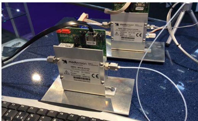
51. Moduvision analytica 2-channel flow, and pressure controller card with user interface software, controls both gas pressure, and flow from an input source, and displays the measured result on PC screen. Email: gvdb@moduvision.com
