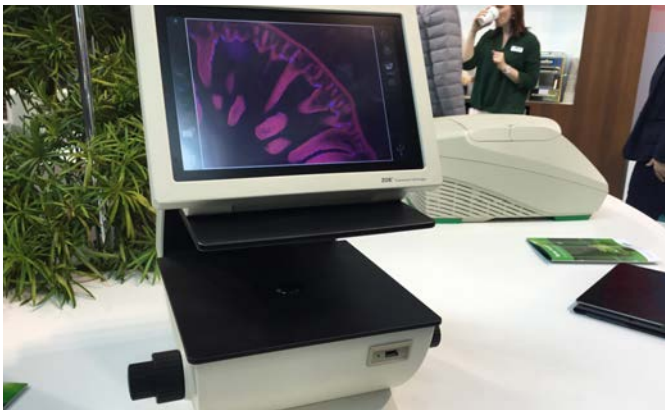
19. Compact fluorescent cell imager allows visualising cells in the desktop. It utilises brightfield and three fluorescent channels to display a wide range of fluorophores. It features touch screen controls: nanette_schlattermund@bio-rad.com
