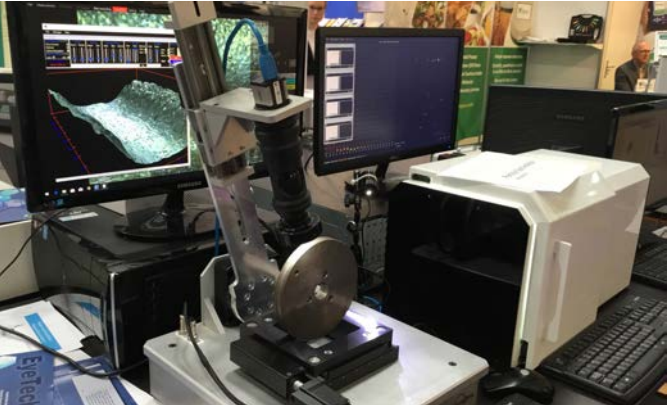
12. 3D digital microscopy by compact MicroOptik allows reconfiguration of its body components to make custom systems. This configuration reveals the surface roughness around a machined disc. Email: havanlieshout@microptik.eu
