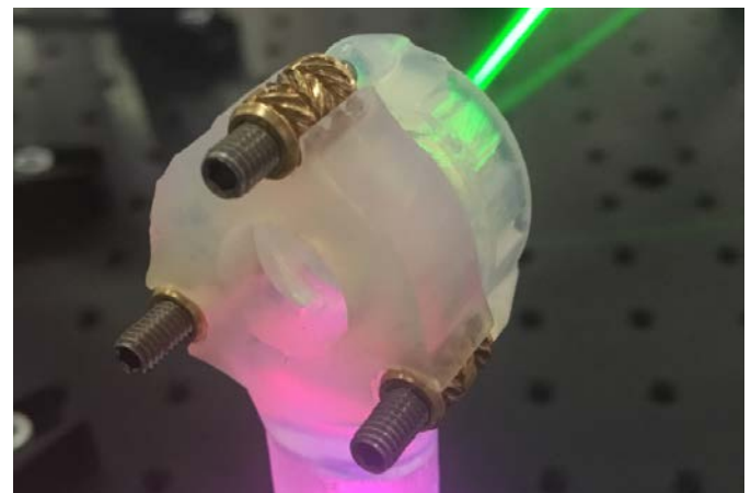
The fine adjustment set screws are secured onto the plastic mount just like the snap-on Microbench rods.
