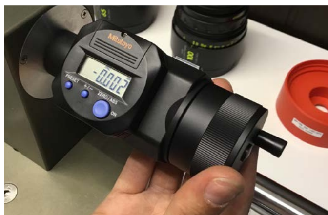
Setting the focus scale of test lens to infinity (left), and the back-focus mirror to zero (right). The non-rotating micrometer spindle has a flat mirror face to reflect back the autocollimator image to its CCD camera for infinity focus check.
