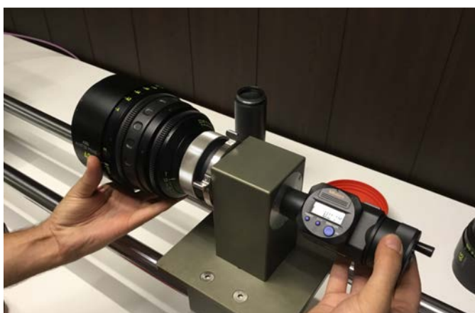
Setting the focus scale of test lens to infinity (left), and the back-focus mirror to zero (right). The non-rotating micrometer spindle has a flat mirror face to reflect back the autocollimator image to its CCD camera for infinity focus check.
