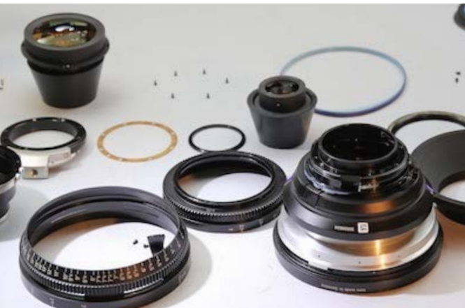
Removing the PL mount on a Zeiss Master Prime lens.
