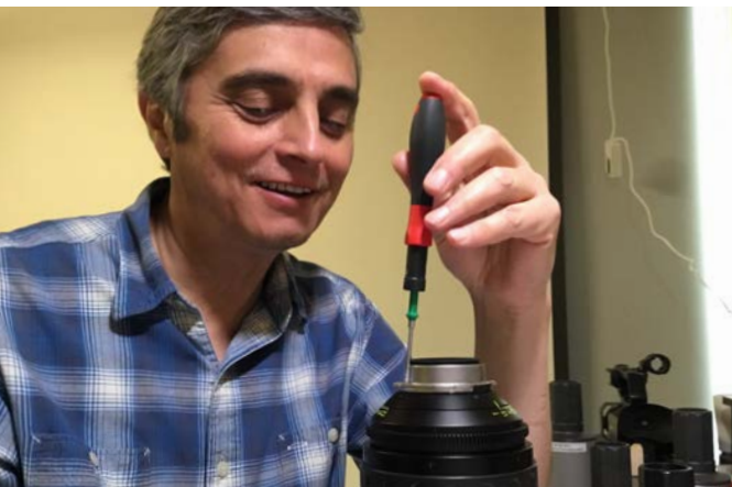
Removing the PL mount on a Zeiss Master Prime lens.
