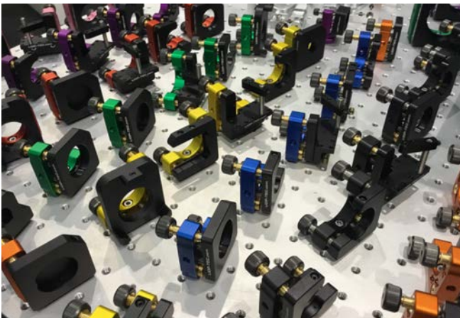
The stage shown above demonstrates the new design approach to large optical mounts to make them lighter, and more compact compared to much bigger, and heavier stages of the past. Precision fiber optics mounts built by Schafter+Kirchoff (above-right) reveals an obsession for rigidity, and precision.
