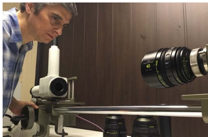
Setting up the Gecko-Cam/Moller Wedel Autocollimator by precise centering of the optical projector with the test lens.
