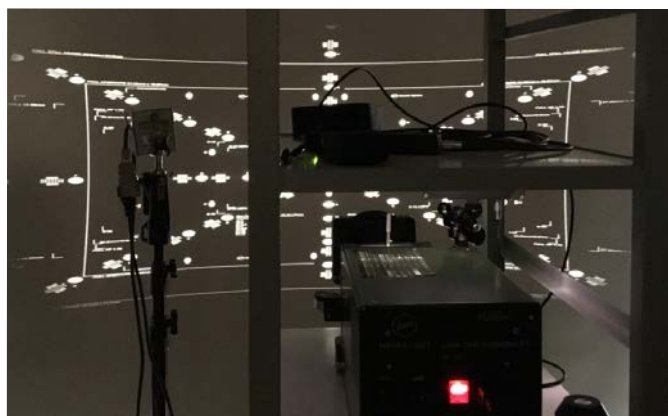
An Anamorphic lens test shows pincushion distortion, and visible chromatic aberration, and defocus on the corners.
