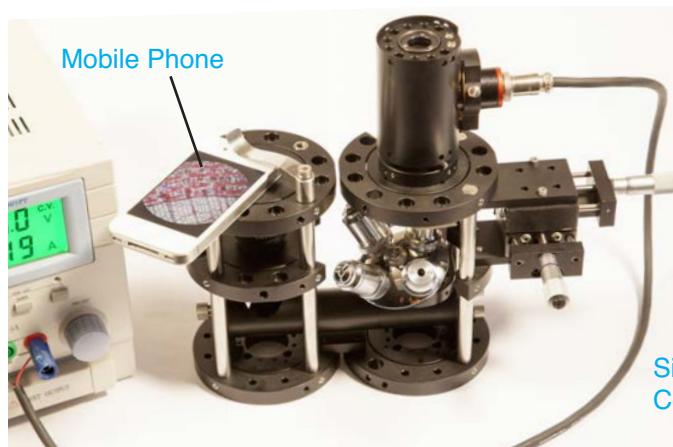
Mobile phone is shown seated above the eyepiece. The image can be centered, zoomed in, and captured.
