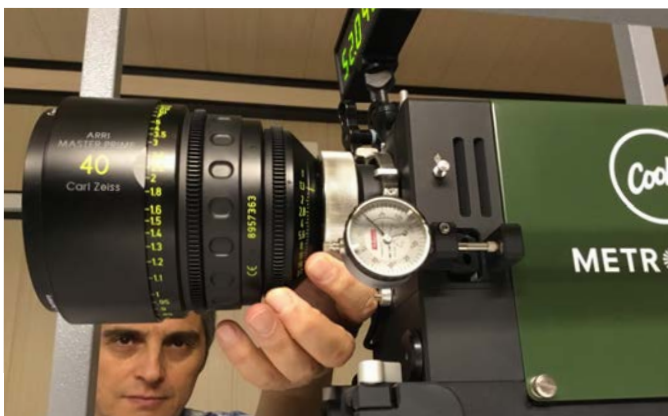
A zeiss Master-prime is installed on Cooke cine projector for direct reading of its lines of resolution, and contrast.
