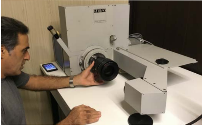
Hossein Jalili testing a Zeiss Master Prime lens with Carl Zeiss tester to verify its MTF performance at PD Cine.
