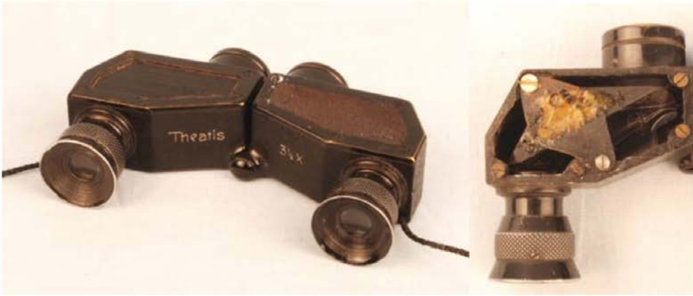
Lemman prism binoculars (theatis 3.5X; J.D. Moller, Wedel, Germany in late 1920's). Four reflections are obtained with this compact image-errection prism (see below for details). Source: College of Optical Sciences, University of Arizona
