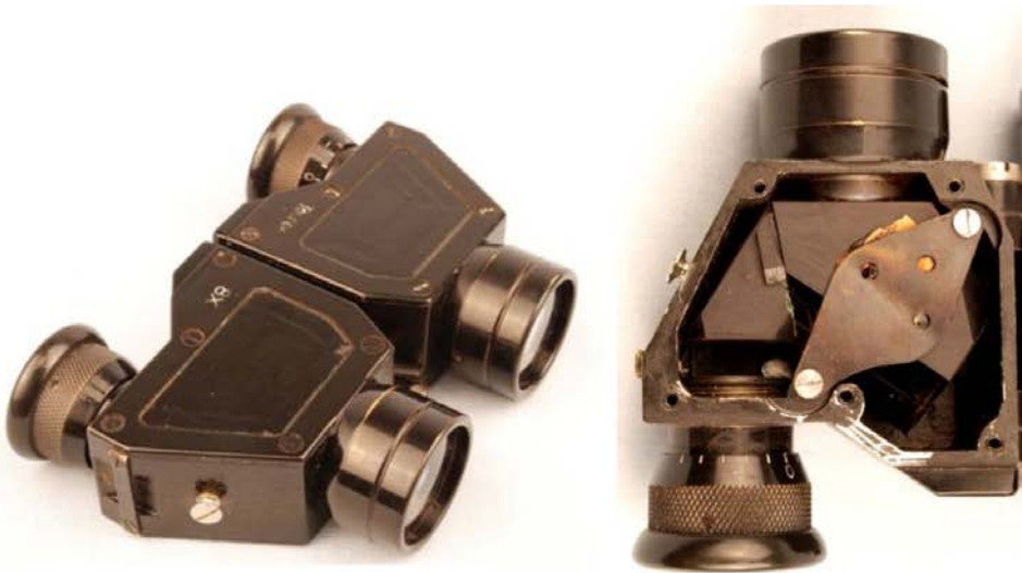
Moller prism binoculars (Tourox 8X; J.D. Moller Wedel, Germany, mid-1920's). This image erection prism system consists of two prisms that are bounded together (right) and held in place by a spring clip. A total of six reflections are obtained. Source: College of Optical Sciences, University of Arizona
