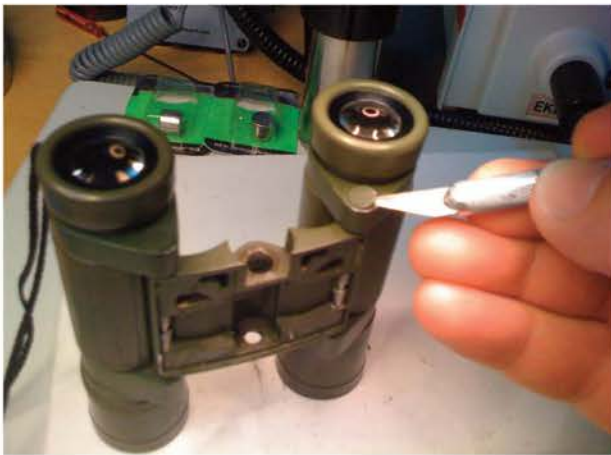
Start moving the cover until it is loose, then remove it using a sharp edge X-Acto knife. The hinge mechanism locking screw is now exposed.
