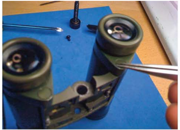
Apply alcohol to the plastic hinge cover. The lock screw is right beneath it.
