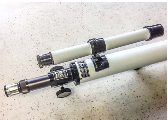
Telescope assembly is straight forward. The singlet glass objective lens is drastically stopped down for color correction.
