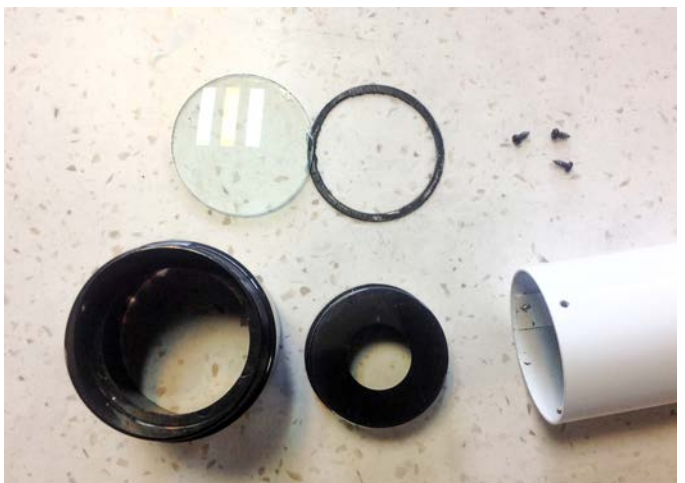
Telescope assembly is straight forward. The singlet glass objective lens is drastically stopped down for color correction.
