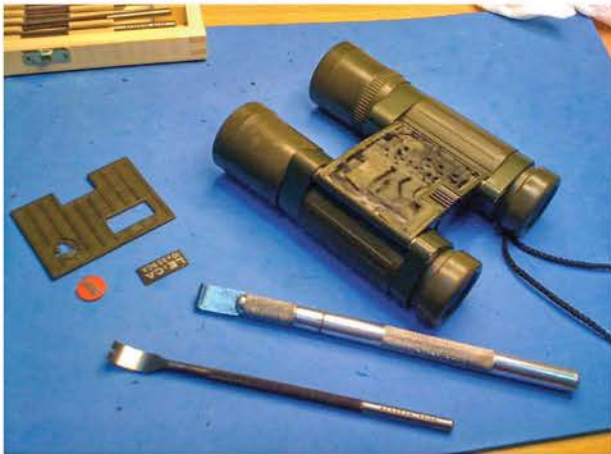
Remove the top cover letherette by a straight edge X-Acto knife. Use alchohol to soften the glue as you progress removing it in small stripes at a time.
