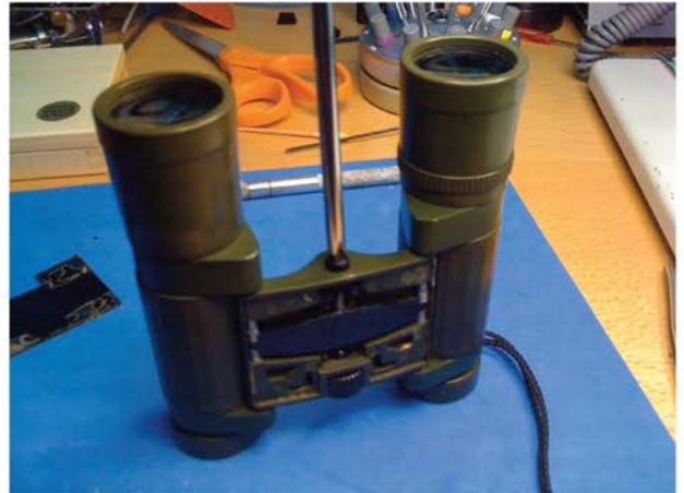
Remove the screw (you need to grab the focusing knob using a 1/8" rubber sheet).
