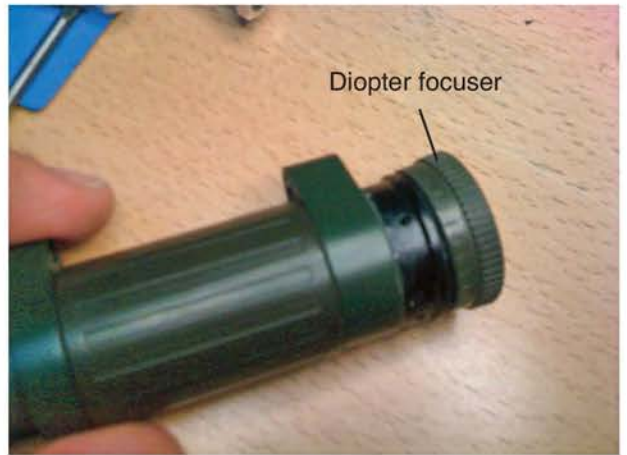
Unscrew, and remove the objective on the other side. Slide off the rubberized diopter focuser from its metal ring.
