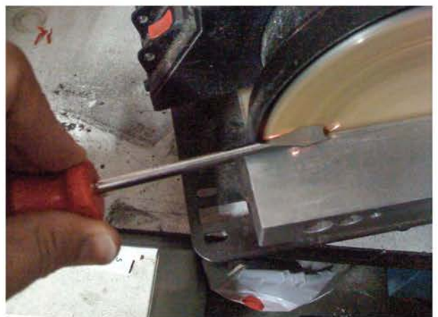
Sand off the outer edge by rotating the entire screw-driver blade. Sand it down slightly less than the diameter of lock screw.
