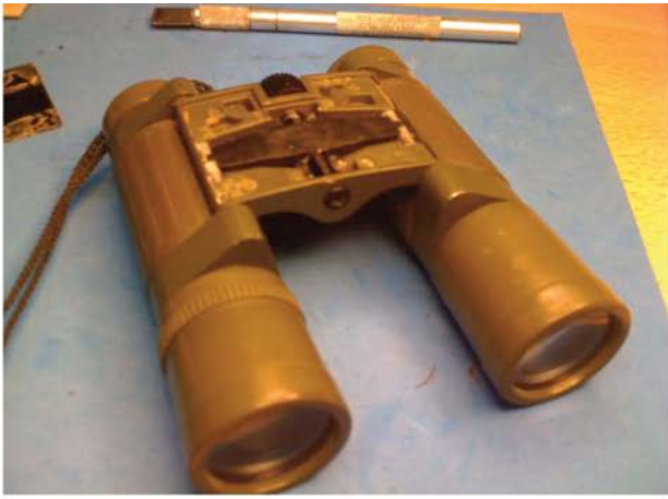
Next step is to remove the focusing knob screw. This is loctited in place.
