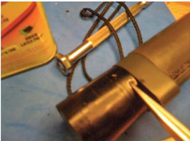
Use tweezers to apply the solvent. This screw rotates freely after it is loose. So it can't be taken out unless the nut is held first on the other side.
