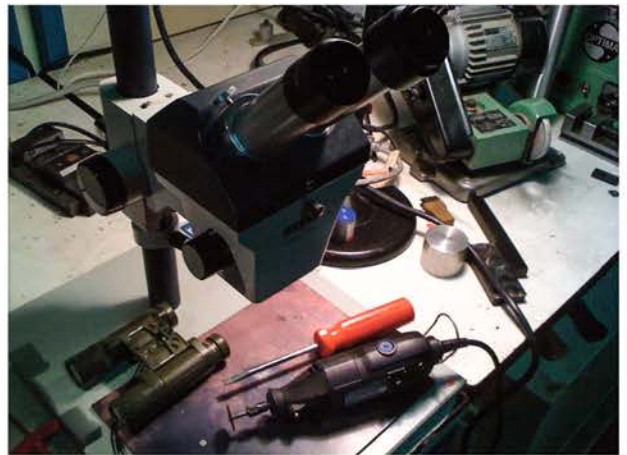
It's time to make a special tool. You need a Dremel with a cut-off wheel attached, and a flat-edge screw driver to sacrifice. Work under a stereo microscope.
