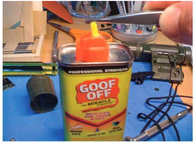
A more powerful solvent can also be used to loosen the screw.
