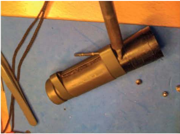
You can heat up the cemented screw via the tip of a soldering iron. This screw secures a guide knot that prevents the focusing lens barrel from rotating.
