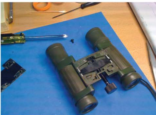
Unscrew the focusing knob, and pull it out.
