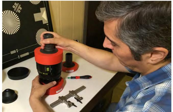
Removal tool for a Zeiss Master Prime frontal lens ring.
