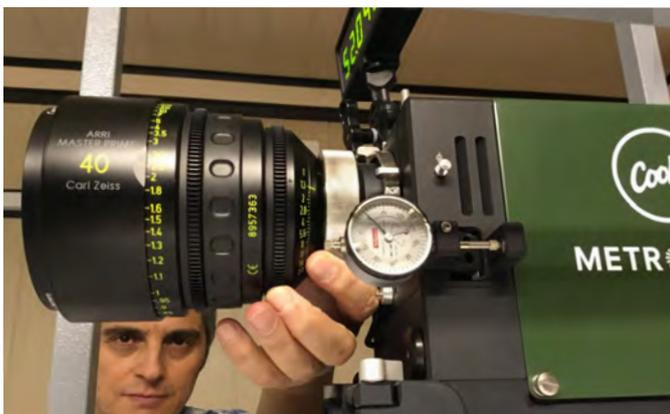
A zeiss Master-prime is installed on Cooke cine projector for direct reading of its lines of resolution, and contrast.
